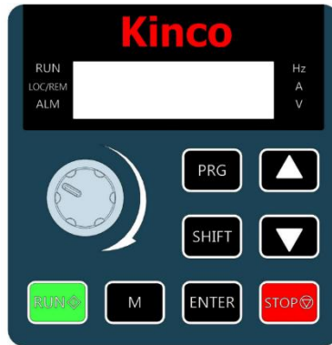
Figure 4-1 Schematic diagram of the LED operating panel
